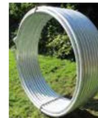
In physics, a sound tube is used for measuring the duration of an echo, for example. A ten metre long plastic tube is fitted with a microphone at both the ends. If you burst a small balloon at one end, the sound will travel back and forth several times. Up to 17 echoes can be detected in one second. The speed of sound can therefore be calculated as  $17 \times 20 \text{ m/s} = 340 \text{ m/s}$ .
